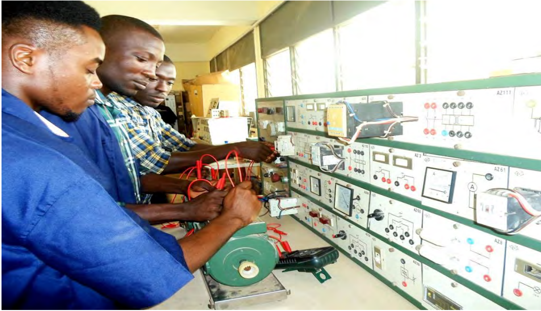
Figure 4.4: Students testing an electric motor to verify its electrical properties after it has undergone maintenance (rewinding) while the researcher observe.
