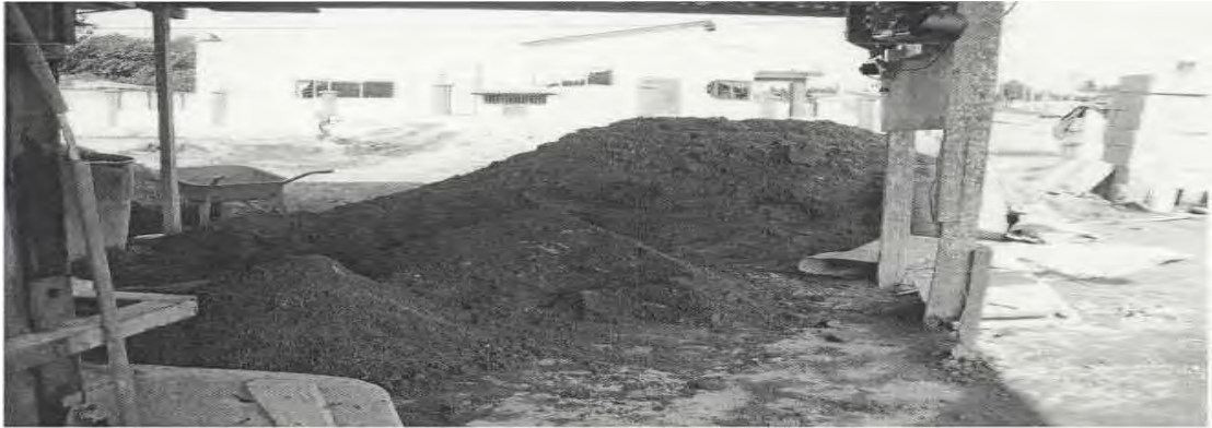
Plate 6: A mixture of cement and sand ready to be moulded into precast sandcrete blocks.
