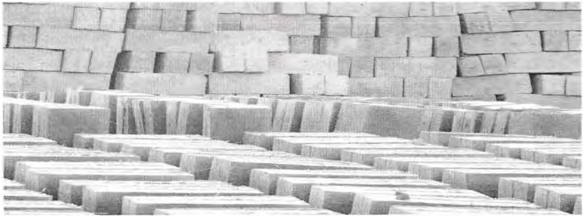
Plate 8: Precast sandcrete blocks being cured after which it is packed and stored/stacked in the open air.
