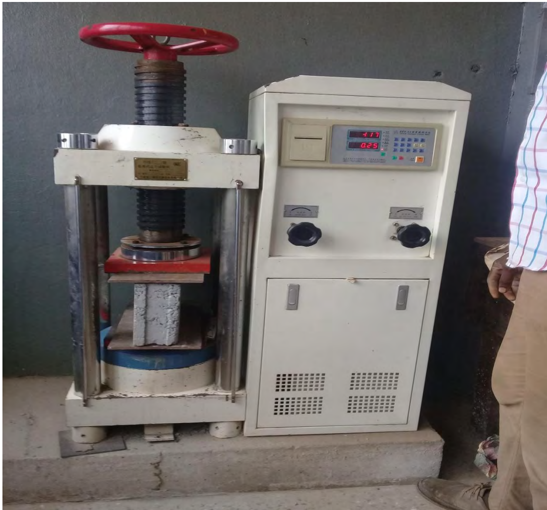
Plate 5: Crushing test being conducted on a sandcrete block to determine the compressive strength.
