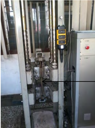
Fig. 3.5: Computer Controlled Universal Testing Machine.
