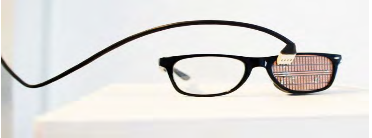
Figure 2. 2 : Spectacle with an Eye Blink Sensor, ( https://www.google.com.gh ).
