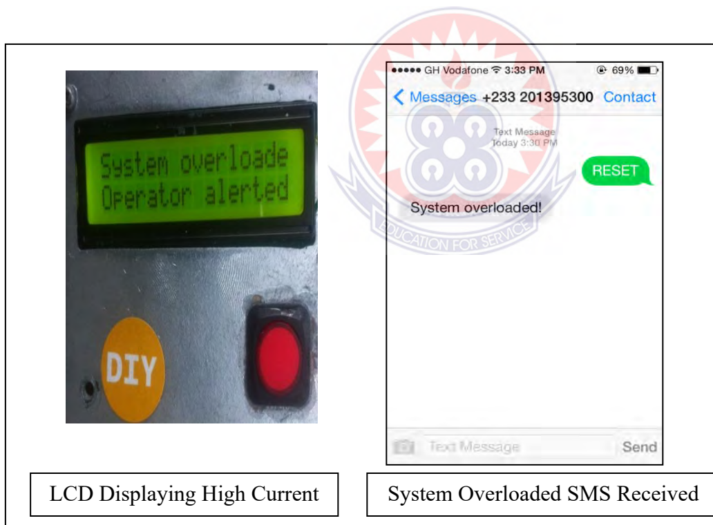
Figure 5.2: System Reporting Overload
