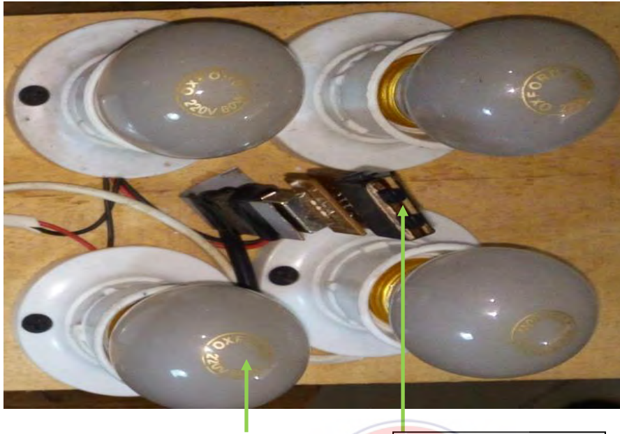
Figure 4.2: Connection of 60W Incandescent Bulbs and Temperature Sensor
