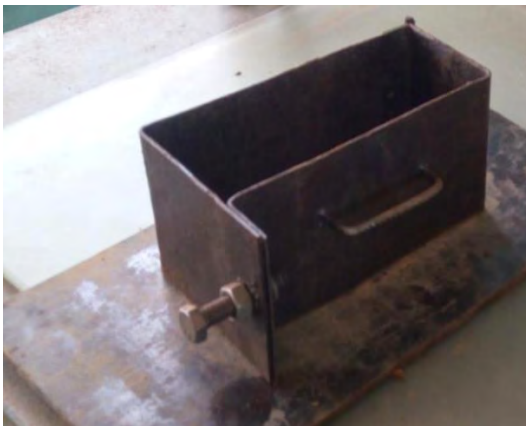
Figure. 3.20 Improvised Moulding Equipment
