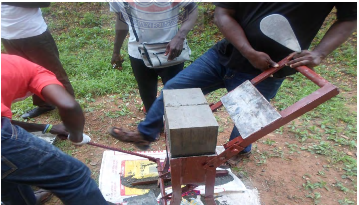
Plate 3. Removing of the composite from the mould box
