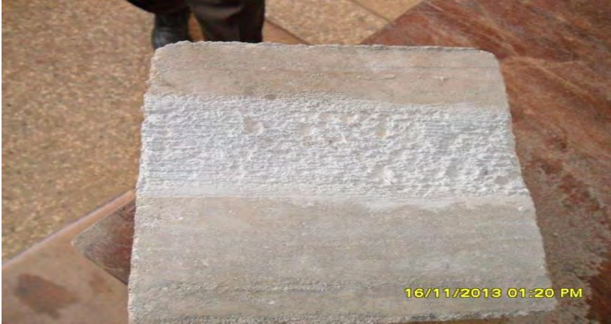
Figure 3.7: Sample cube after abrasion test
