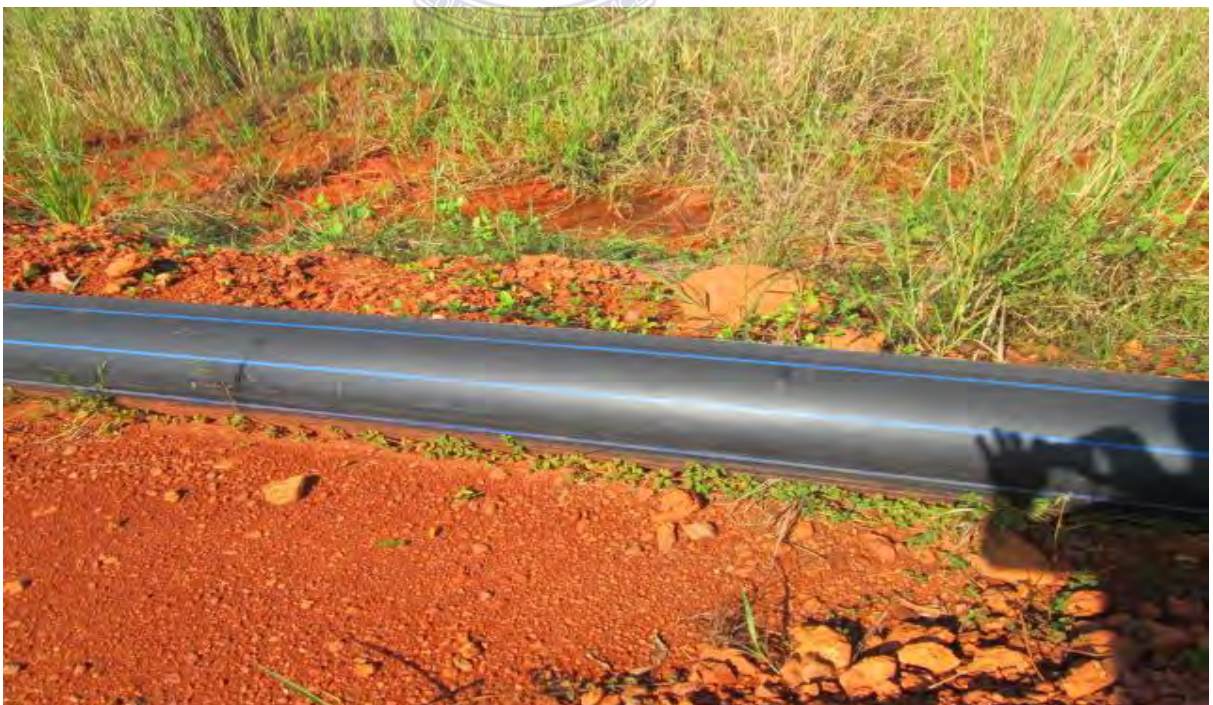
Plate (ii) pipe carrying the slurry from washing plant to the disposal point
