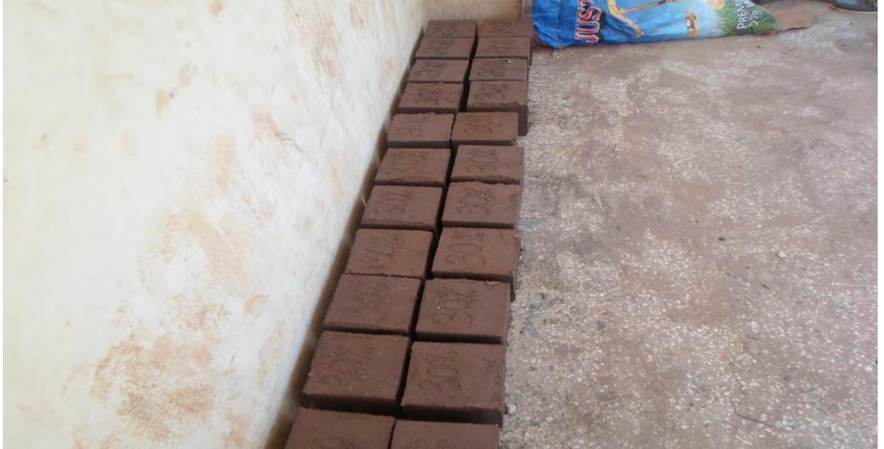
Figure 3.4 Curing of composite cubes
