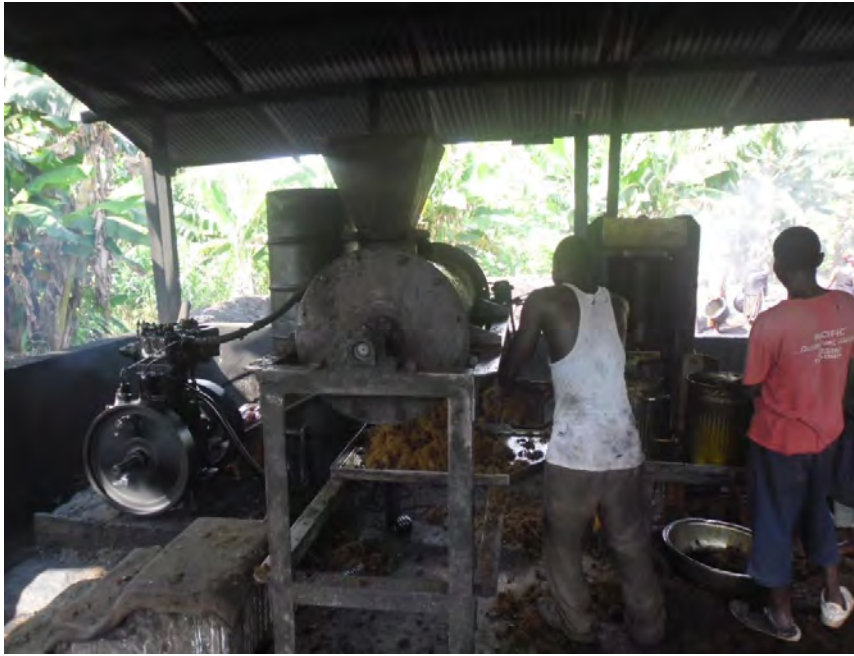
Figure 13: Photograph Showing the Use of a Digester and a Hydraulically Hand Operated Press to Process Palm Oil
