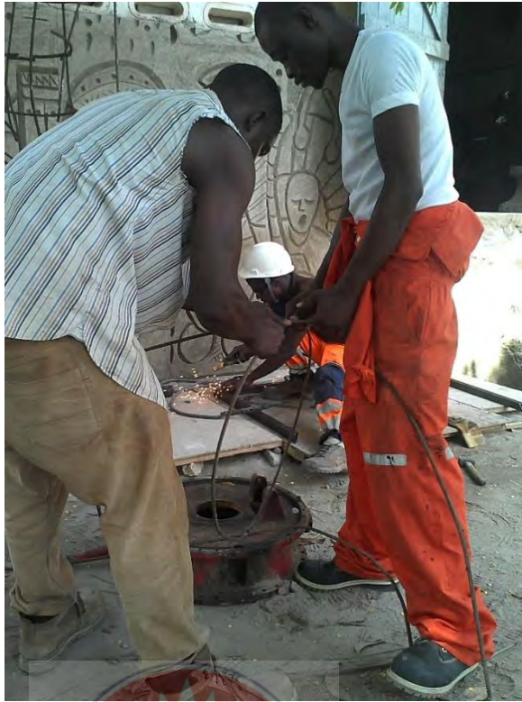
Figure 5.11(F) Curling and perforating of metal base for iron rod
