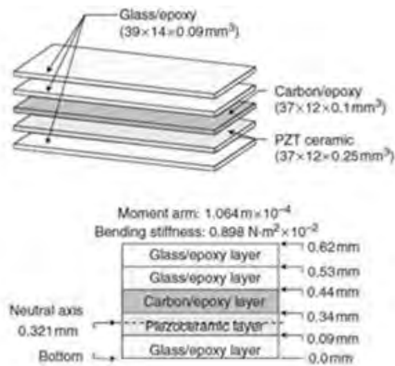
Figure 8: Geometry and position of the neutral axis of PCGE-A (Elfrink et al. 2009)
