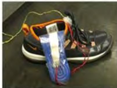
Figure 9: A piezoelectric film-based power generator. (Mateu et al. (2006)
