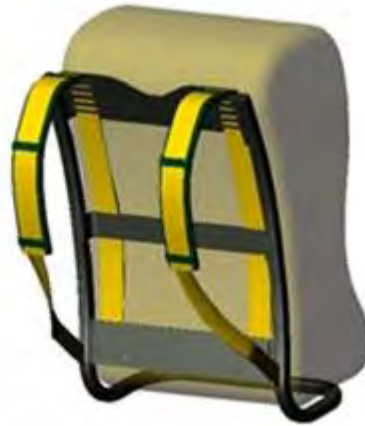
Figure 10: Schematic of the backpack with piezoelectric straps. (Farinholt et al. 2007)
