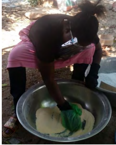
Figure 58: Mixing Colouring Oxide with powdered glass
