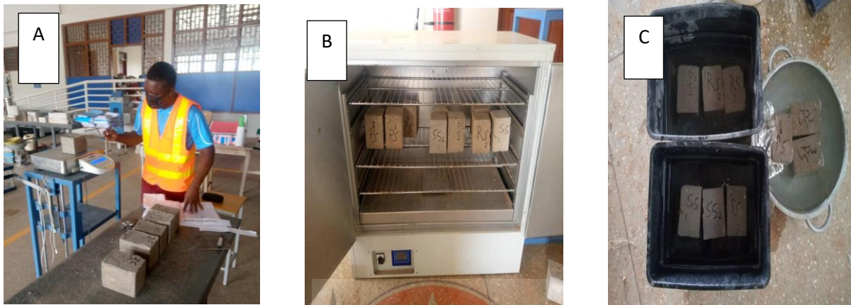
Figure 3. 8: Determining the water absorption
