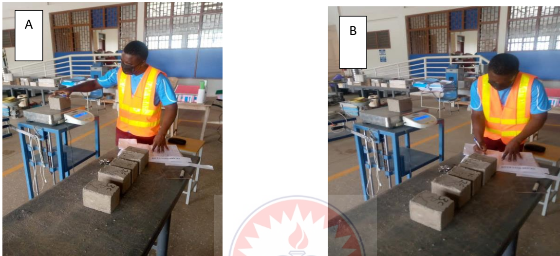
Figure 3. 7. Determining the density test
