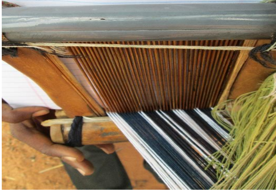
Plate 3.3: Denting of the Warp for Fugu weaving
