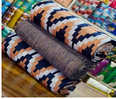
Plate 4.11: Kente cloth showing both design and plain weave with pattern warp
