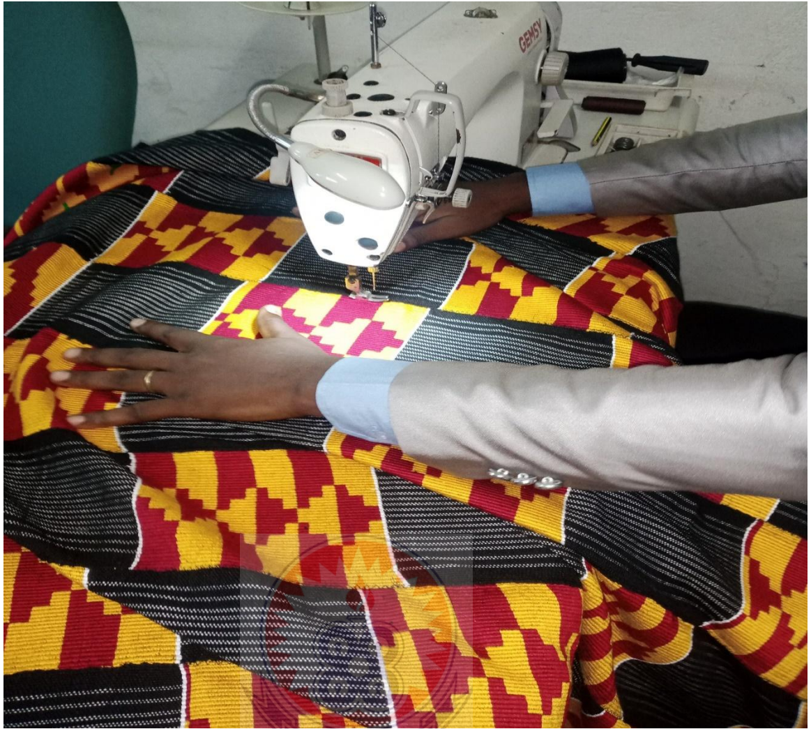
Plate 4.33: Joining of innovative woven strips.
