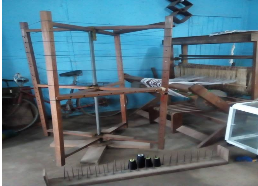
Plate 4.15: Doubling and twisting of yarns Source: Researcher's Fieldwork, 2022.
