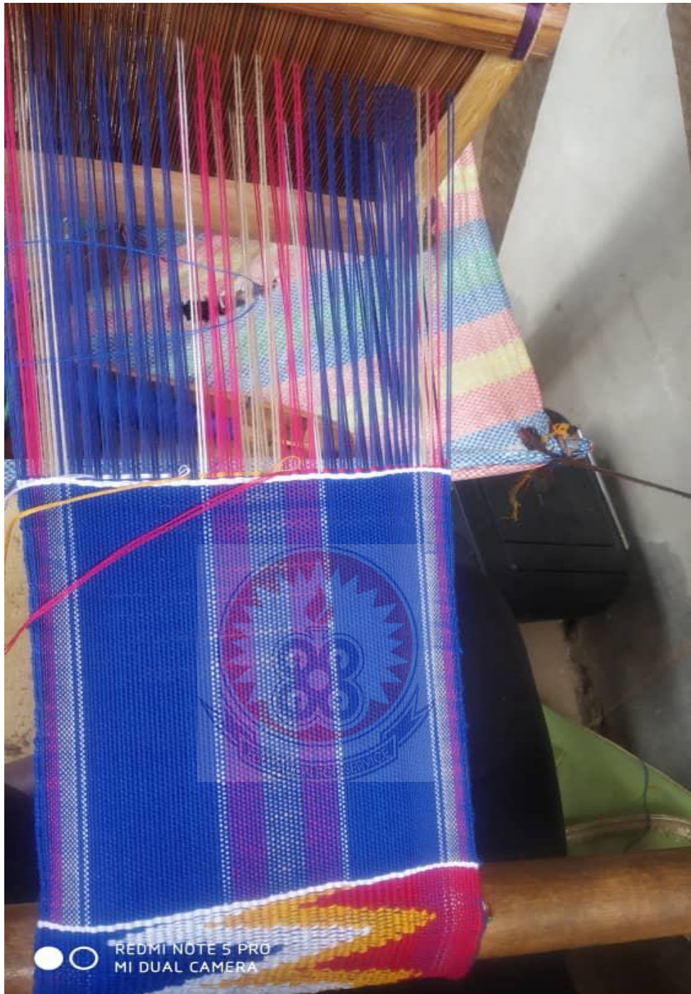
Plate 4.23: Weaving process of the integrated fabric Source: Researcher's Fieldwork, 2022.
