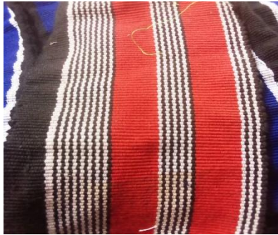
Plate 4.3: A fugu fabric (Saanabodiun) weave with pattern warp
