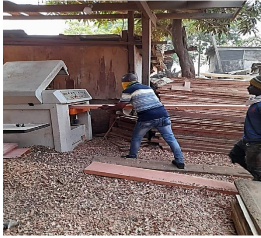
Figure 2.3 The Thickener Machine being fed by timber board at the shop.
