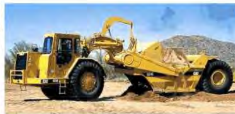
Discharging bowl, spreading soil
