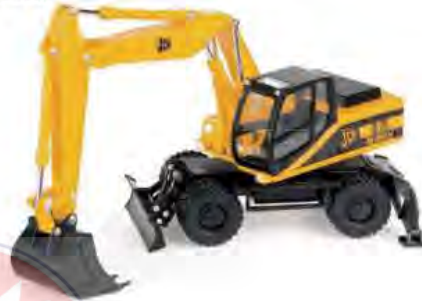
Wheel-mounted backacter slewing excavator
