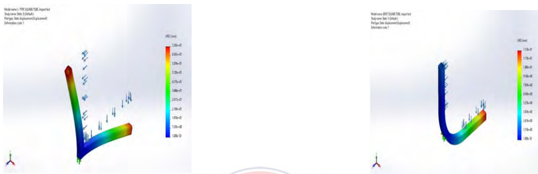
(a) Displacement model of sample 'L' (a) Displacement model of sample 'C'
