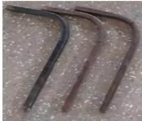
Figure 3.11 Prepared Bent sample shape Specimen for tensile test (Specimen B)
