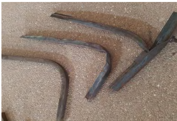
Figure 3.13 failed curve welded shape specimen
