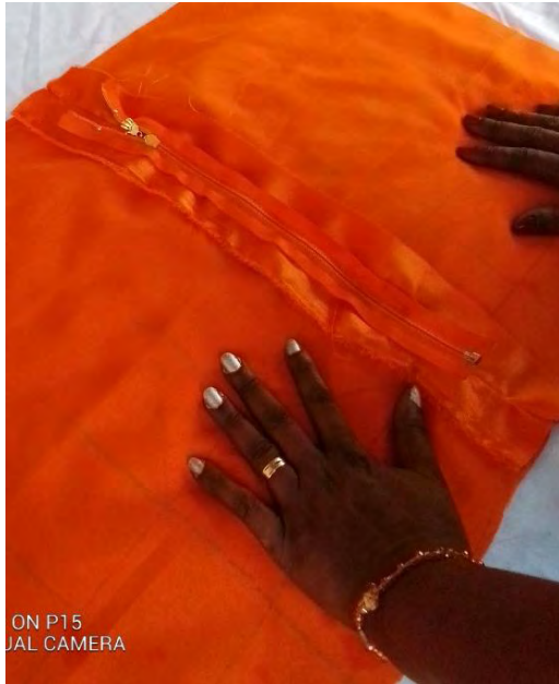
Plate 4. 14: Zip at wrong side
