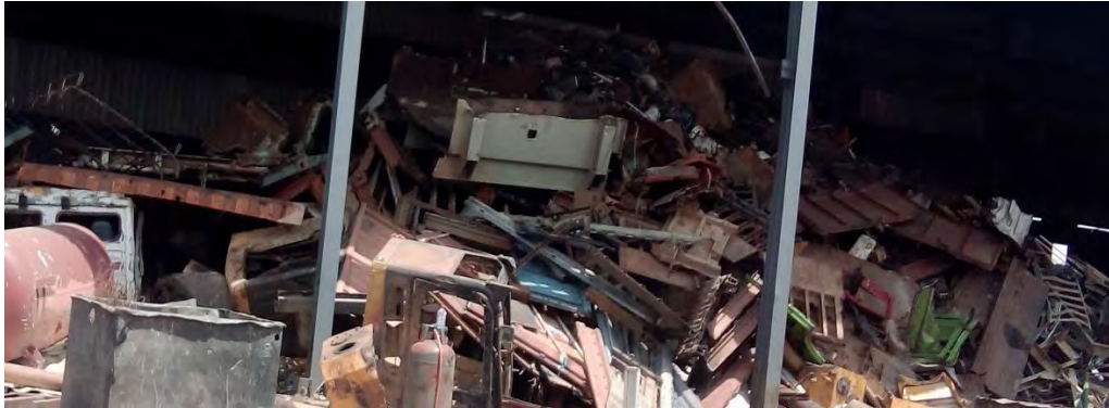
Figure 2. 4: Collected scrap used for rebar production in Ghana
