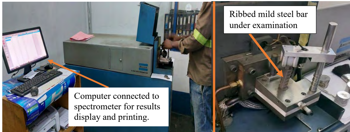
Figure 3. 3: Angstrom V-950 Spectrometer for Chemical Composition
