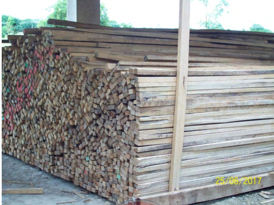
Fig 4.13: As observed, timber packed in dampness and not on wooden stickers
