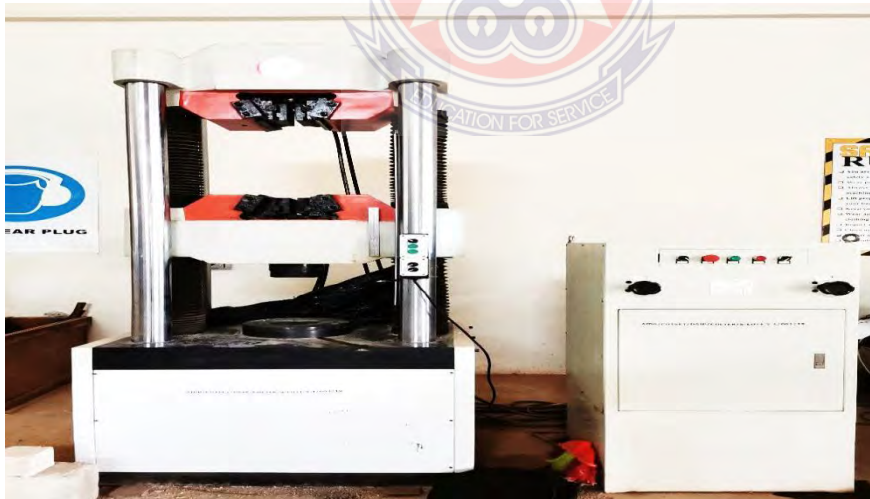
Figure 3.7 Universal testing machine – model WAW-1000H
