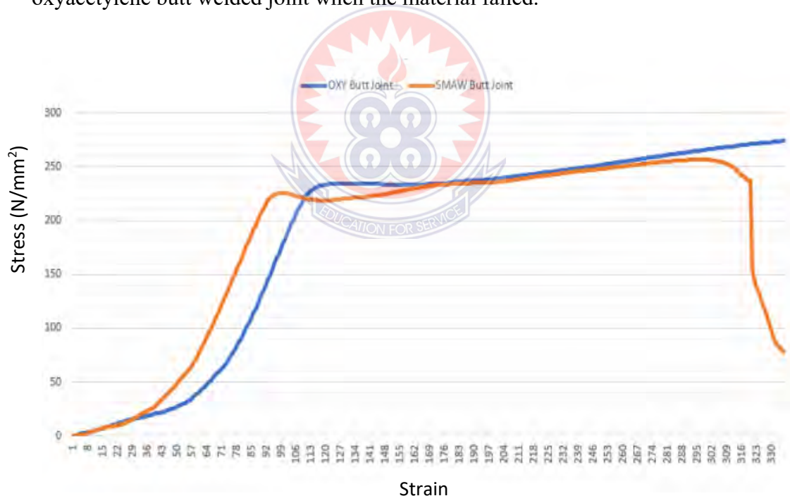
Figure 4.5 Stress-Strain for Butt Joint
