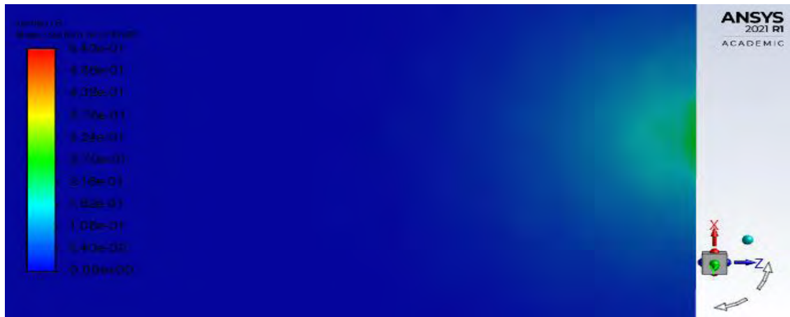
Figure 4.25: Contours plot of Octane Mass Fraction of single GDI
