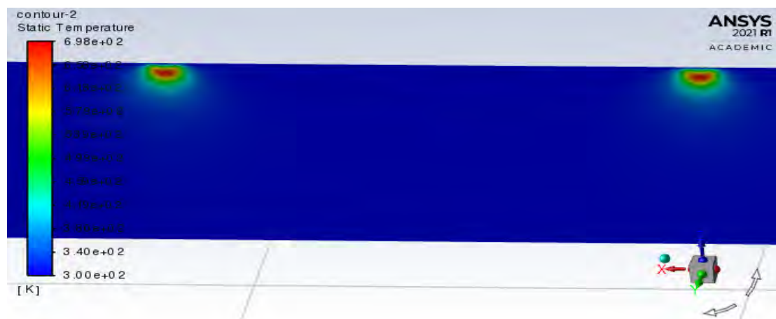
Figure 4.13: Contours plot of Temperature distribution for Variable Cp of dual GDI
