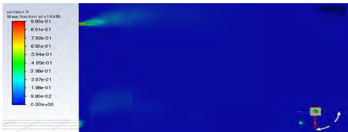
Figure 4.26: Contours plot of Octane Mass Fraction of dual GDI
