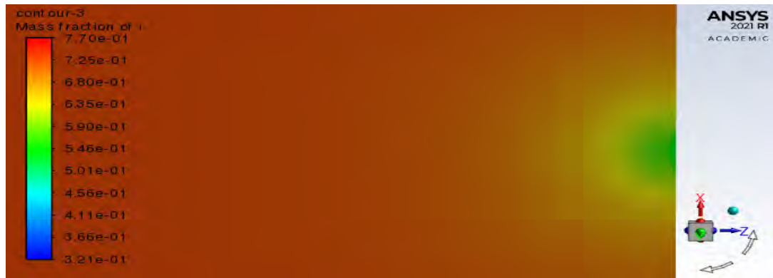
Figure 4.37: Contours plot of Nitrogen Mass Fraction of Single GDI
