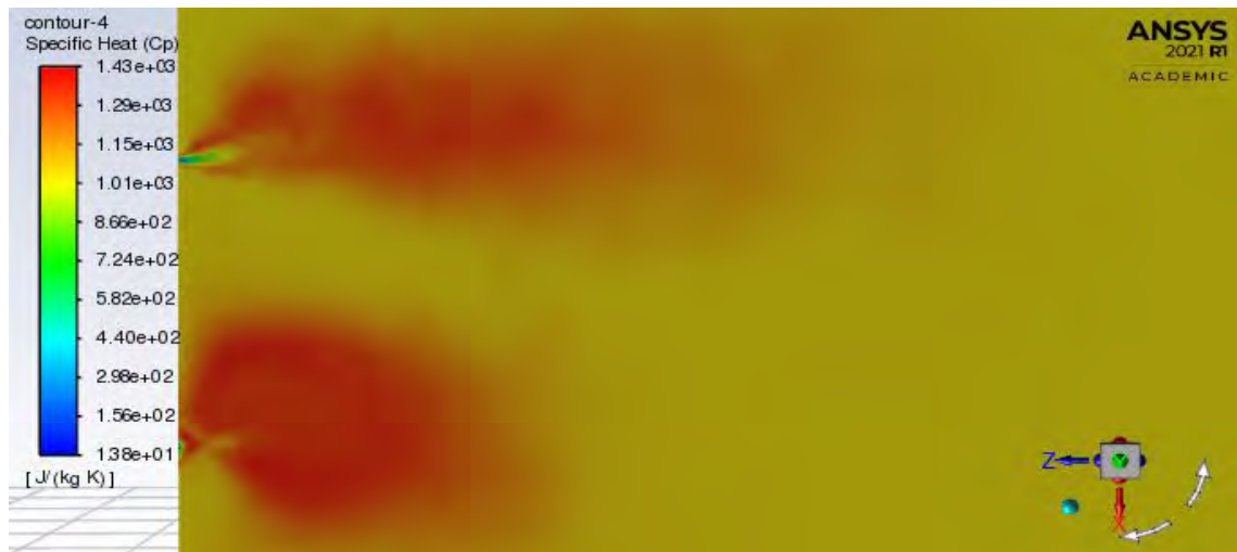
Figure 4.15: Contours plot of Temperature distribution for Specific Heat of dual GDI
