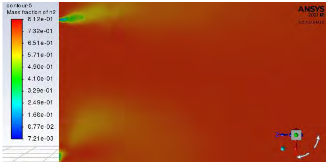
Figure 4.38: Contours plot of Nitrogen Mass Fraction of dual GDI
