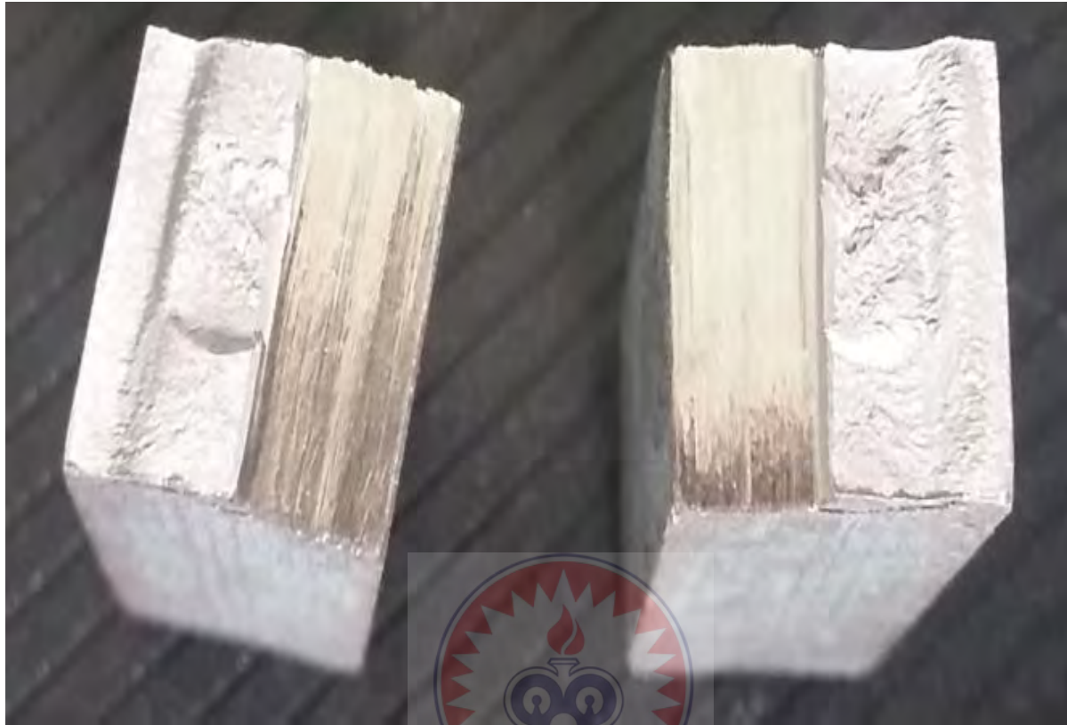
Figure 5.5.3 Fracture Surface after Impact
