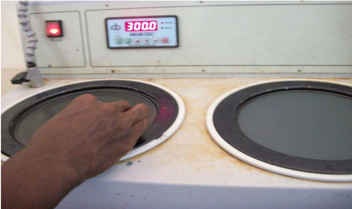
Fig. 3.2 Labpol Duo and Twin disc machine for polishing samples for testing (enlarged). 20 th September 2012. Source: Physics Department – KNUST, Kumasi.
