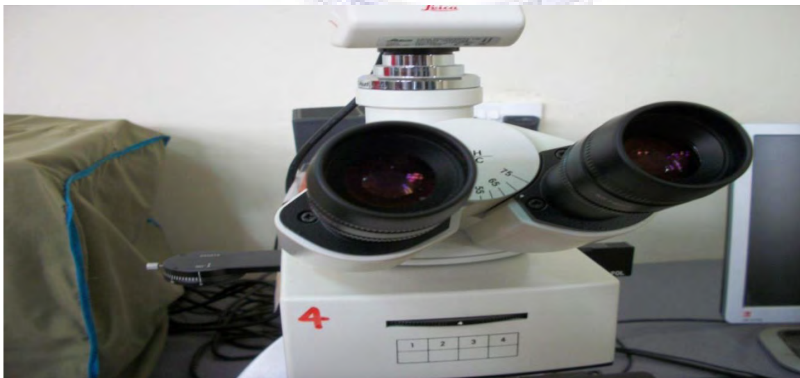
Fig. 3.3 Lecia DM 1000 Machine for checking microstructure of samples (enlarged). Source: Physics Department – KNUST, Kumasi.
