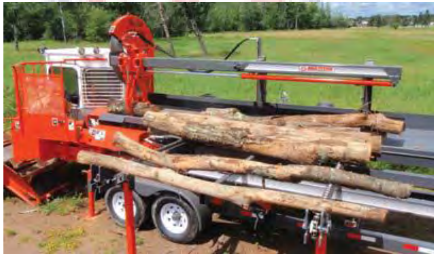
Figure 2.1. Multitek 2025- a mobile bandmill used in sawing small-diameter logs.
