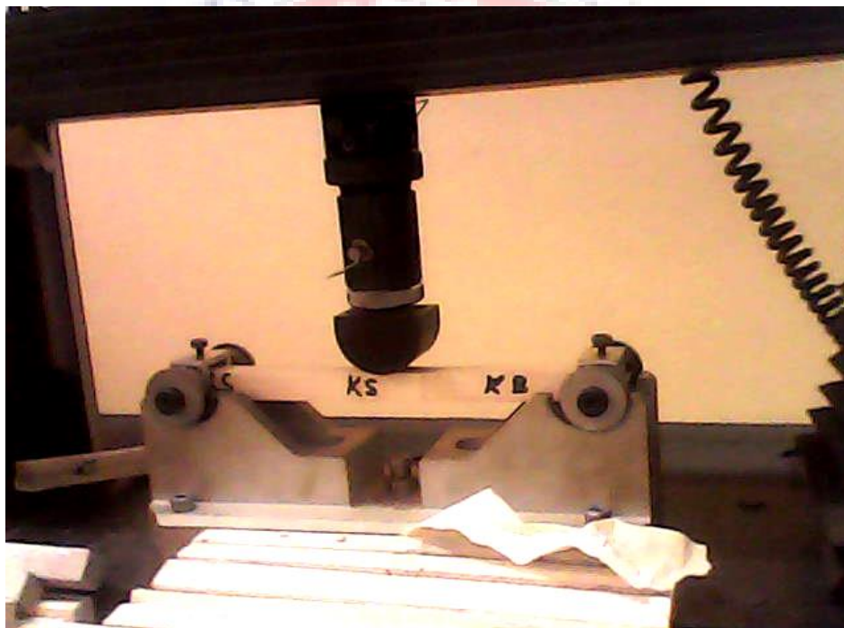
Figure 3.9: Bending strength test set-up for testing both solid/unjointed and finger-jointed lumber in the INSTRON machine showing some of the samples under test.
