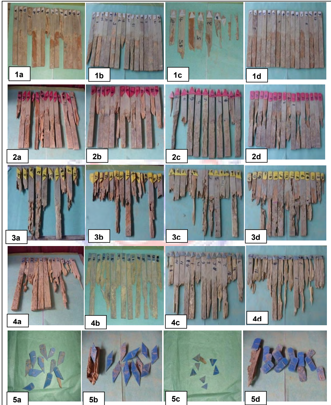
Figure 4.2.2. Appearances of the remains of Stem and Branch Wood `samples after Durability Test {1= E. cylindricum ; 2= E. angolense ; 3= K. ivorensis ; 4= T. superba ; and 5= P. macrocarpa }; a = stemwoods (MC1), b = Stemwoods (MC2), c = Branchwoods (MC1), and d= branchwoods (MC2) of the various species}. The control specimens ( C. pentandria ) were not tagged and all were destroyed.
