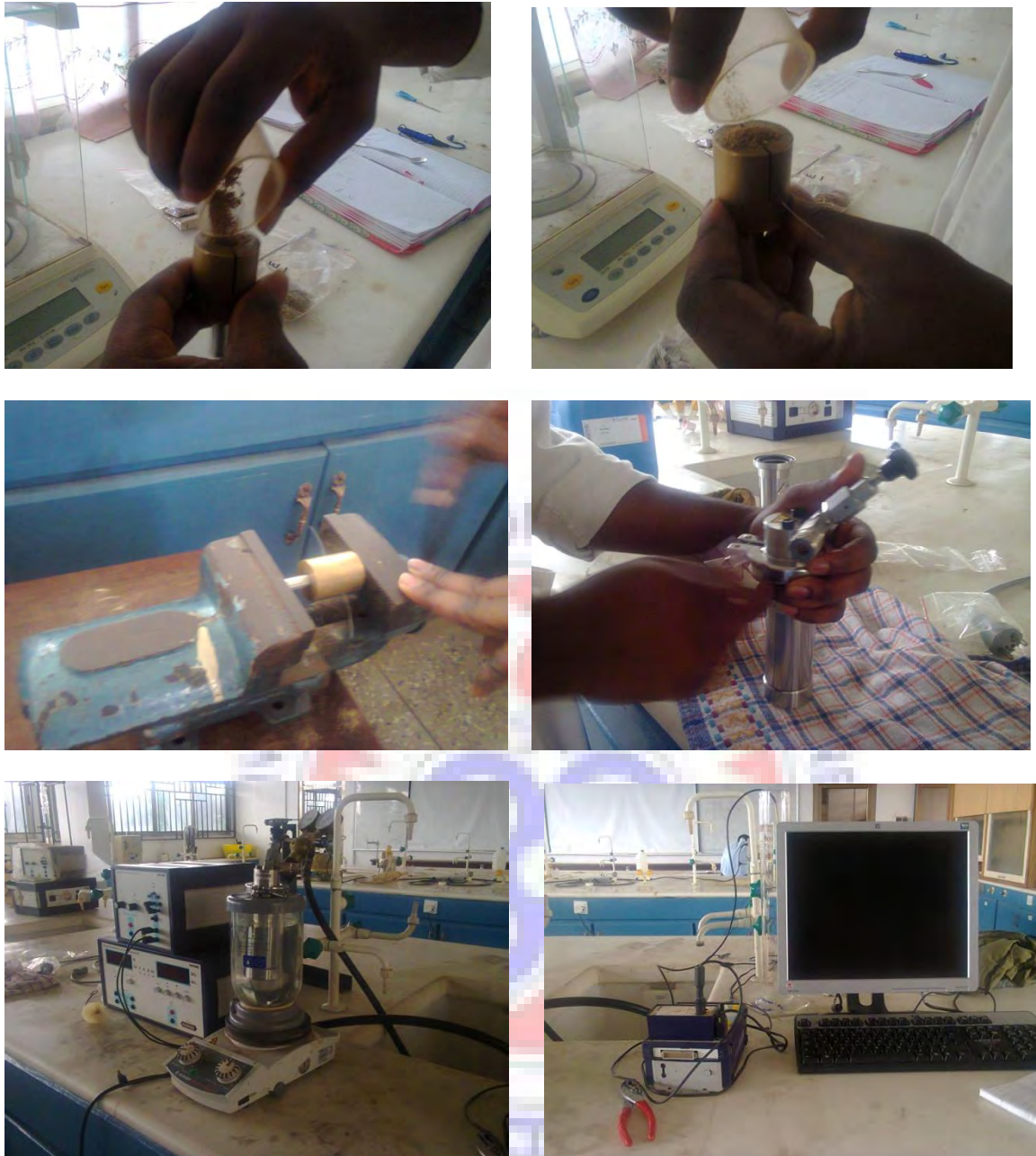
Plate 3.5 Determining the Calorific values of the bamboo samples using Bomb Calorific
