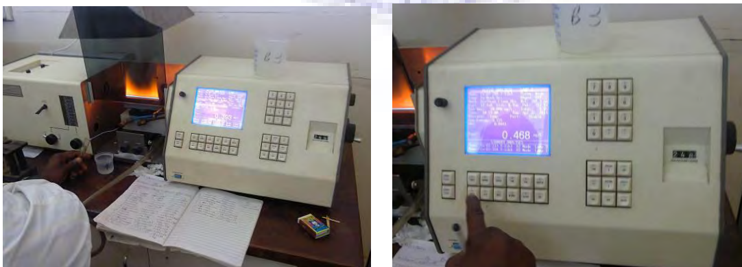
Plate 3.8 Determining Ash elements using Atomic Absorption Spectrograph (AAS)
