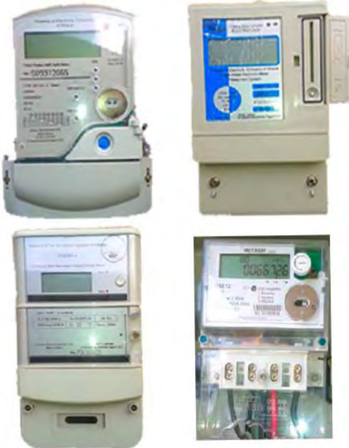
Figure 3.1: Standalone Prepaid Energy Meters Deployed by ECG
