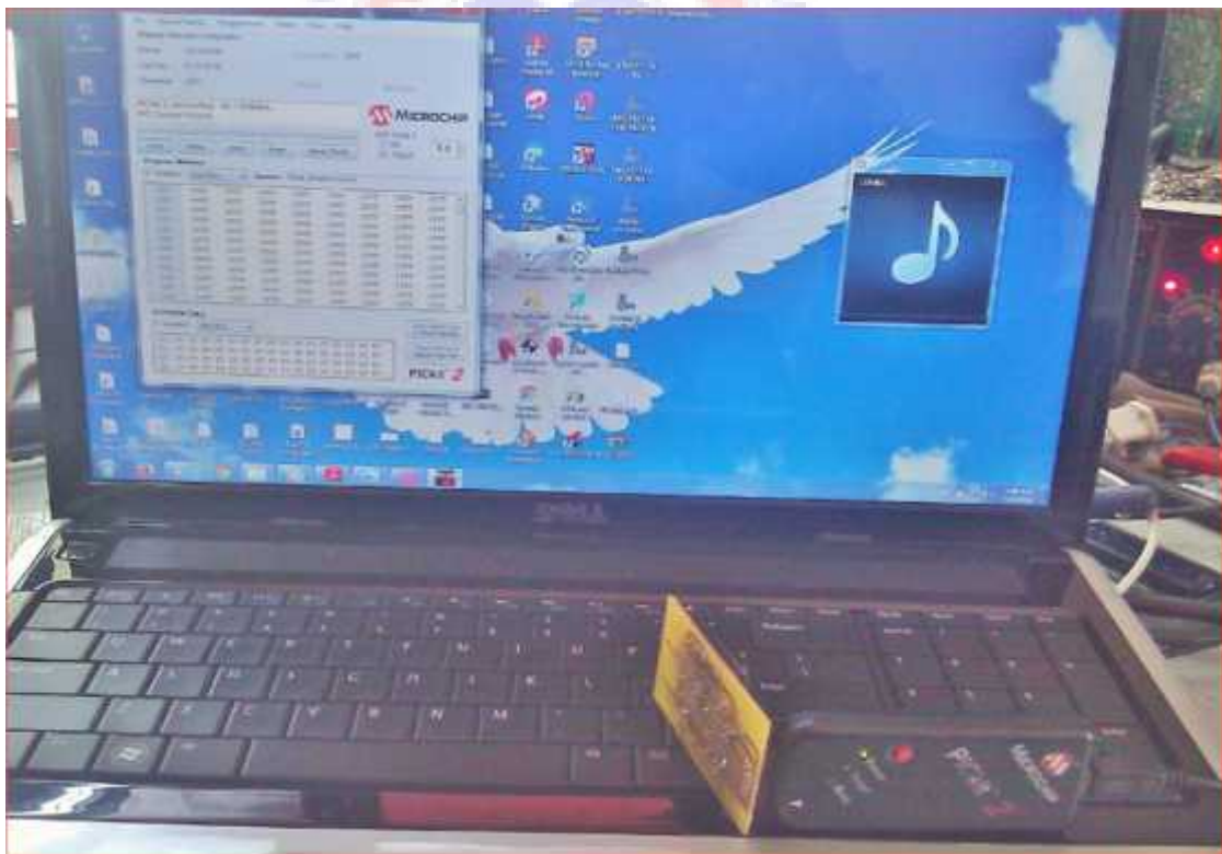
Figure 3.13: The setup interface for loading HEX file from the computer into microcontroller Pic 16f84 using microchip Pic kit2.
