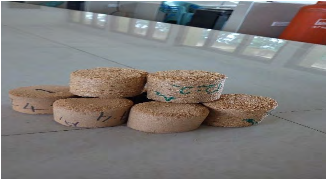
Sample of the Celtis briquettes used for the smoking of the fish
