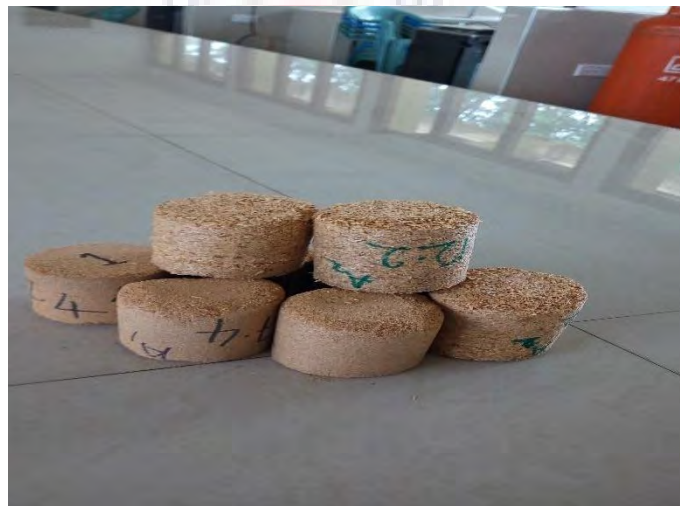
Figure 4.1: Sample of the Celtis briquettes used for the smoking of the fish
