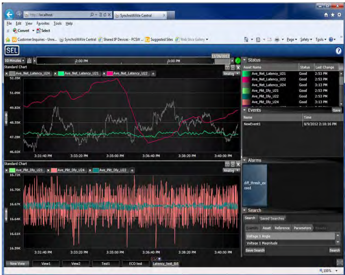
Figure 3.9: Synchrowave displaying the average network latency of PMU on the upper half of the screen and average interpacket latency on the lower half of the screen.
