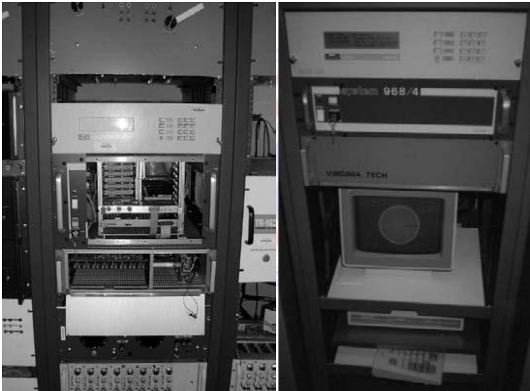
Figure 2.1: First prototype PMU built at Virginia Tech
