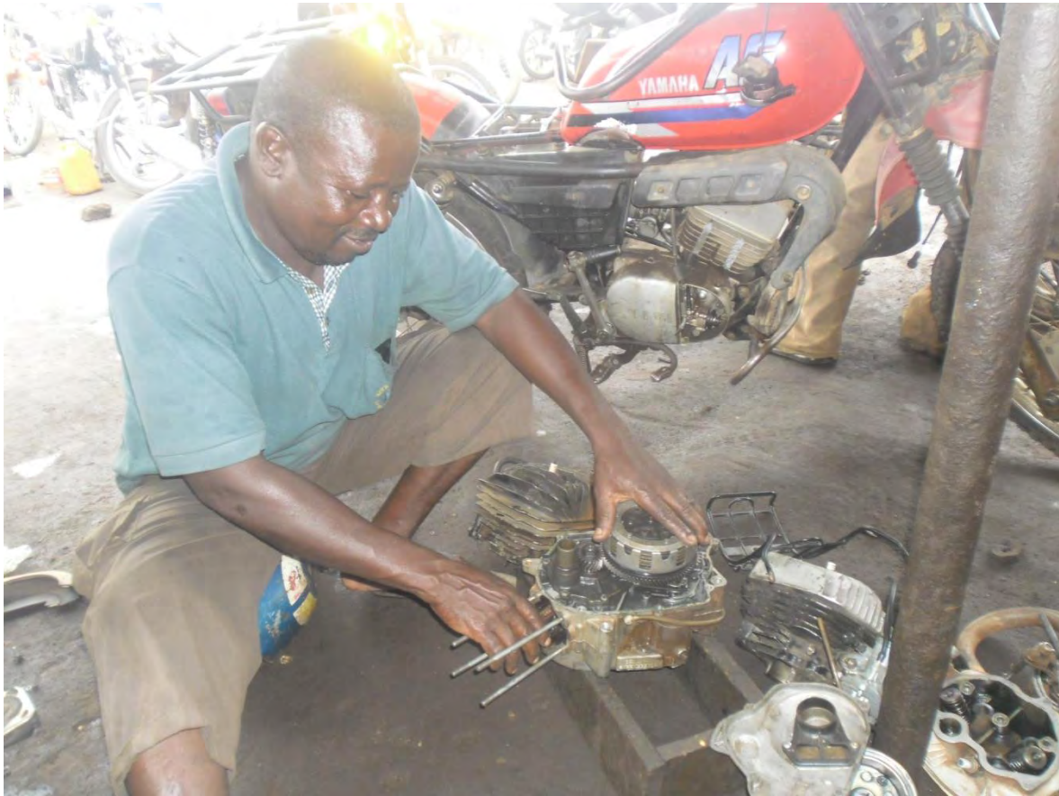
MR. STEPHEN AYINE REPAIRING A GEAR BOX WITHOUT WEARING PROTECTIVE CLOTHING
