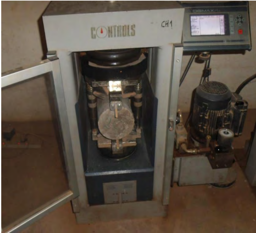
Figure 3.6. Tensile Splitting Strength Testing of Cylindrical Specimen
