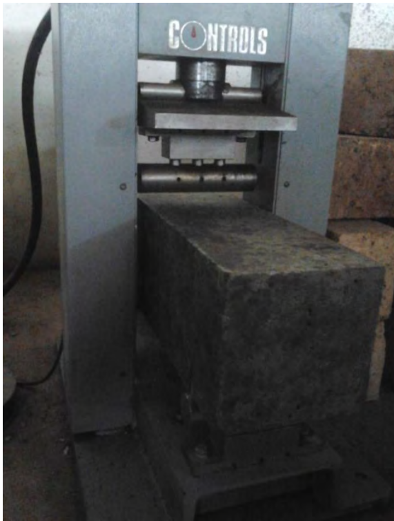
Figure 3.7. Flexural Strength Testing of Beam Specimen
