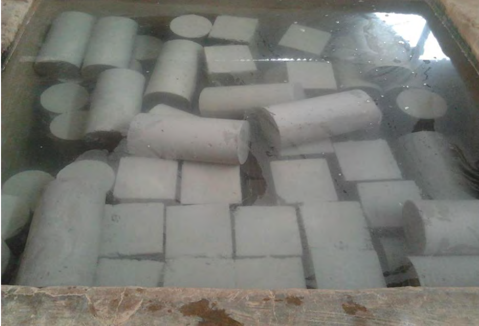
Figure 3.4. Samples of Concrete Specimens under Curing
