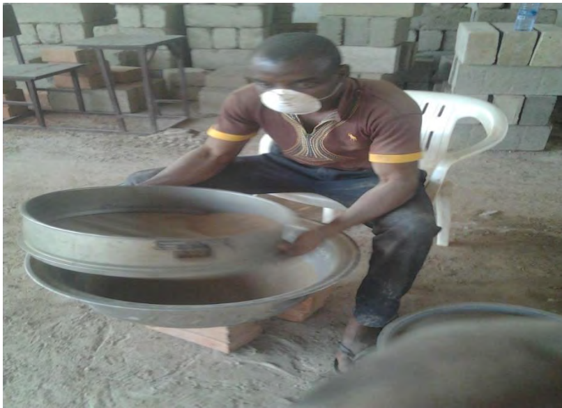
Figure 3.1. Sieving of Fines (Clay/Silt) from Dry Sand
