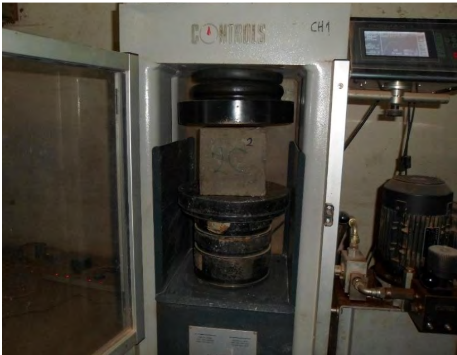
Figure 3.5. Compressive Strength Testing of Cube Specimen
