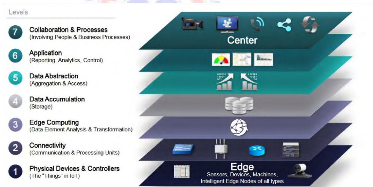
Figure 3: IoT reference model: Source; Cisco systems 2014
