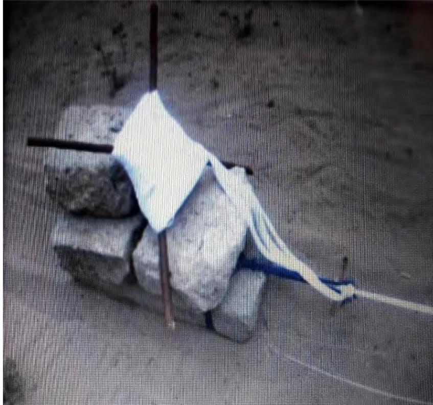
Figure 9: Stretched warp ends attached to dragstone Source: Field Work Data (2018)
