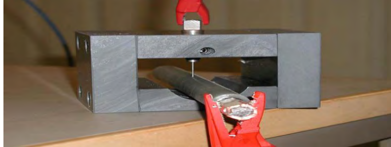
Figure 14: Cable (Needle) test set up
