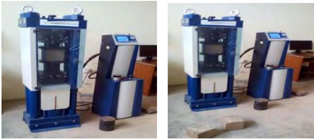
Figure 3.5: Automatic Tensile and compressive machine CSIR-BRRI Civil Engineering Laboratory Source: Researcher Field construct 2018
