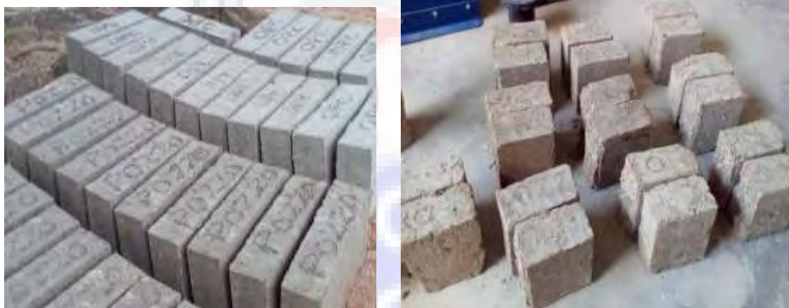
Figure 3.6: The sample specimen pozzomix cement and OPC sandcrete blocks for the crushing test at BRRI-CSIR Civil Engineering Laboratory Source: Researcher Field construct, 2018
