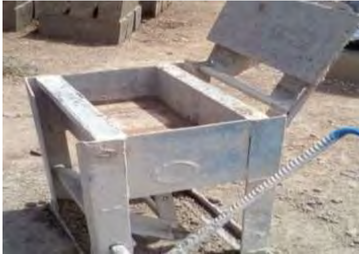
Figure 2.4: Manual block moulding machine at Ave Maria concrete products-Tanoso, Sunyani Source: Researcher Field Construct, 2018
