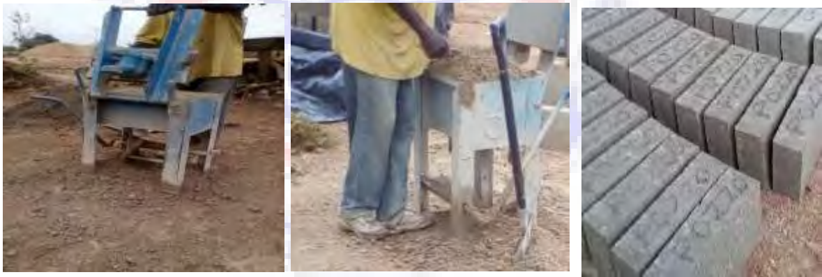
Figure 3.3: Pressing of cement and sand mixture in the manual moulding machine to manufacture pozzomix cement and OPC sandcrete blocks at Aprade construction site Source: Researcher Field construct 2018
