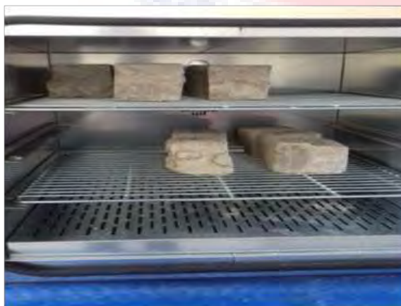
Figure 3. 8: Oven for curing pozzomix cement and OPC sandcrete blocks for water absorption test at CSIR-BRRI Civil Engineering Laboratory
