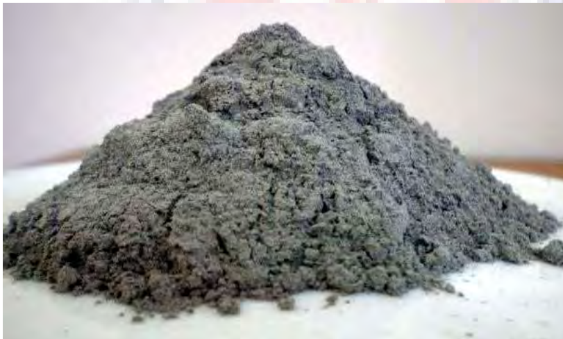
Figure 2.7: Fly ash from BRRI material laboratory Source: Researcher Field Construct, 2018
