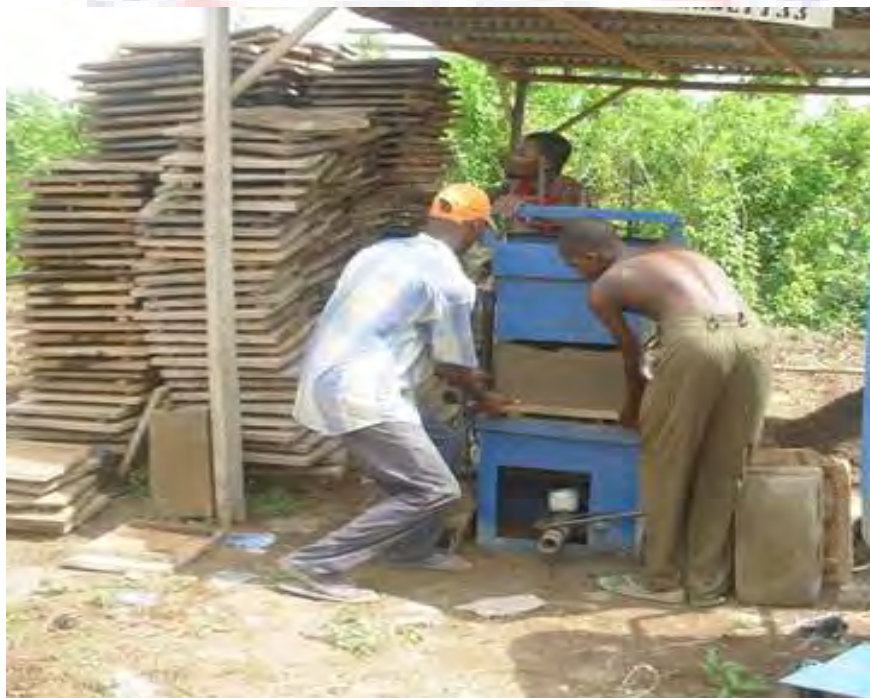
Figure 2.3: Automated block moulding machines from Ave Maria concrete products-Tanoso, Sunyani Source: Researcher Field Construct, 2018
