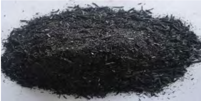
Figure 2.9: Rice husk ash from BRRI material laboratory
