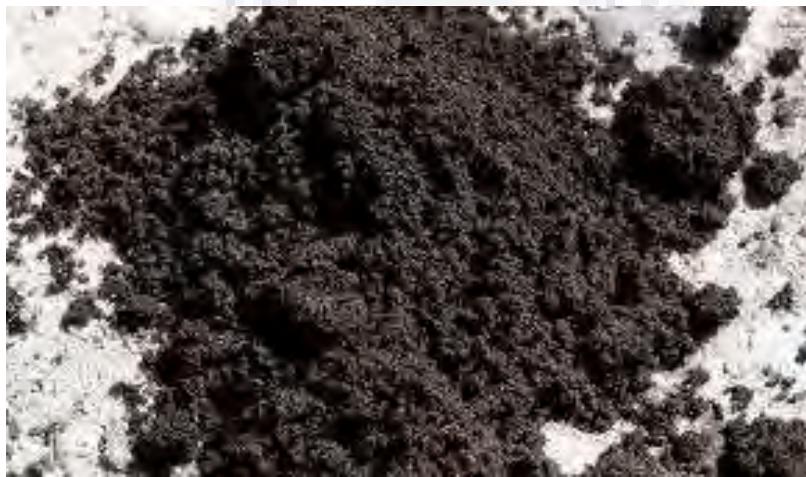
Figure 2.6: Volcanic ash pozzolana at BRRI material laboratory
