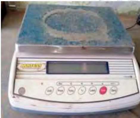
Figure 3.7: Digital balance for measuring pozzomix cement and OPC sandcrete blocks prepared for water absorption test at CSIR-BRRI Civil Engineering Laboratory
