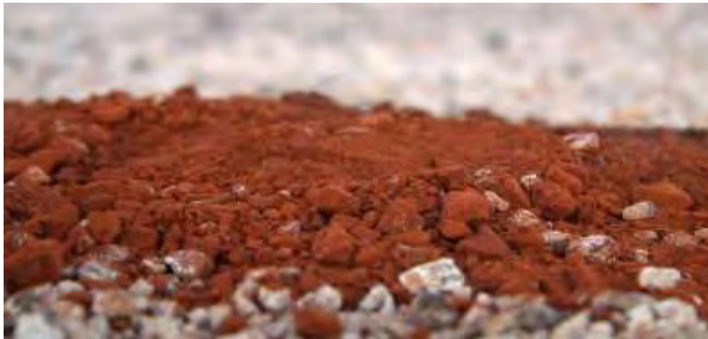
Figure 2.8: Bauxite wastefrom BRRI material laboratory
