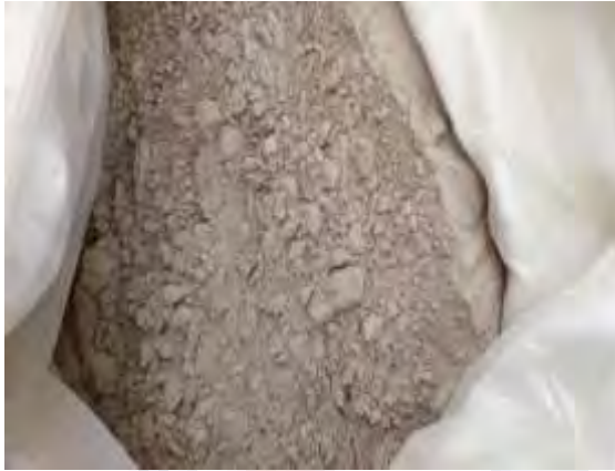
Figure 2.10: Calcined clay pozzolana (now called pozzomix cement) from BRRI material laboratory Source: Researcher Field Construct, 2018
