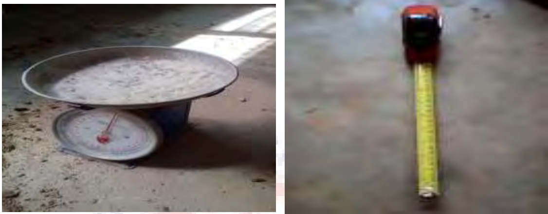
Figure 3.4: Top pan balance and Steel tape measure for measuring the dimensions and weight of pozzomix cement and OPC sandcrete block samples at CSIR-BRRI Civil Engineering Laboratory
