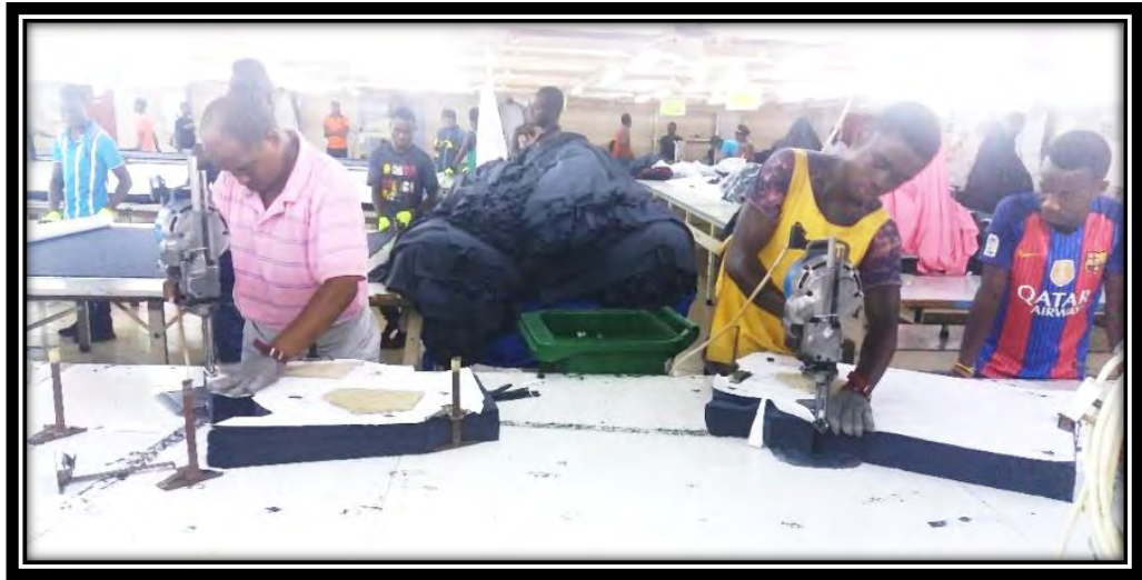
Figure 15: A marker placed on a pile of fabric for cutting Source: Field Research (2017)
