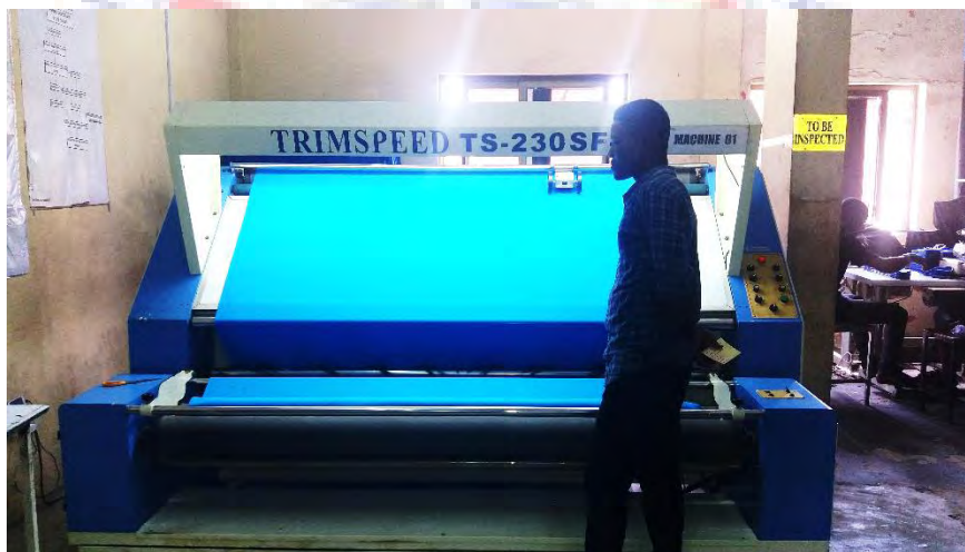
Figure 12: Ten percent of fabric consignment being inspected Source: (Dignity DTRT, 2017)
