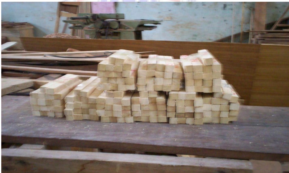
Figure 3.9 A Picture of specimen prepared for turning test of required dimension of 20mm x 20mm x 125mm.
