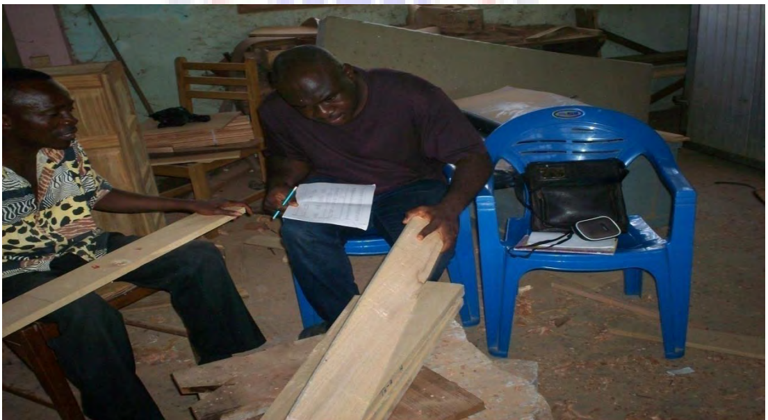
Figure 3.8 A Picture showing visual grading of planed specimen.
