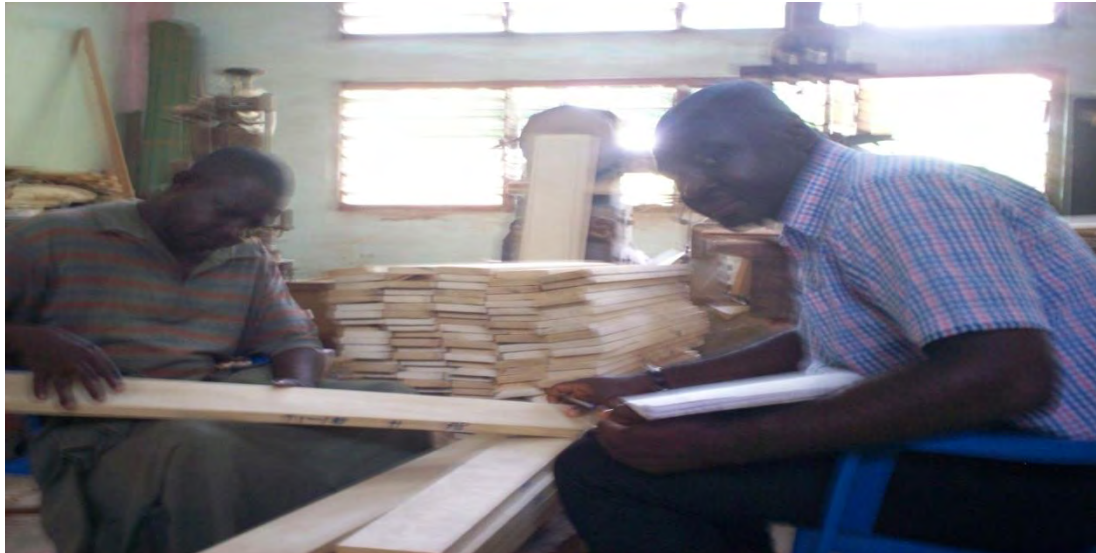
Figure 3.20 A Picture of specimen being visually graded.
