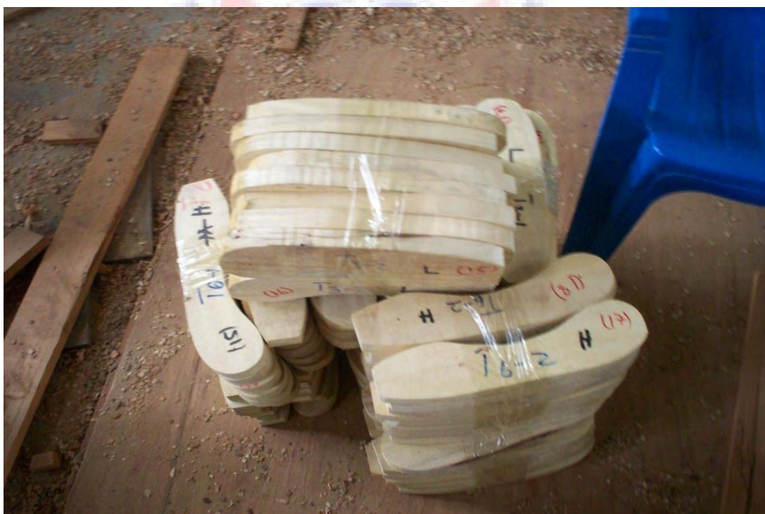
Figure 3.16 A Picture showing shaped specimen ready for grading.
