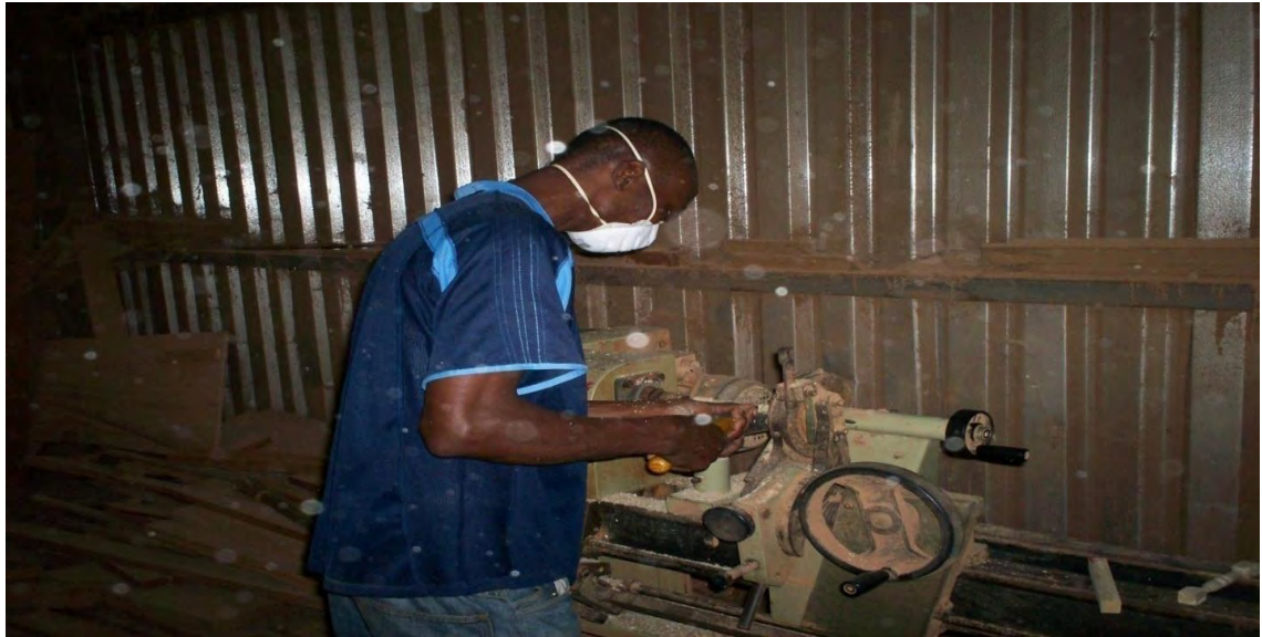
Figure 3.10 A Picture of a sample being turned on the lathe machine.
