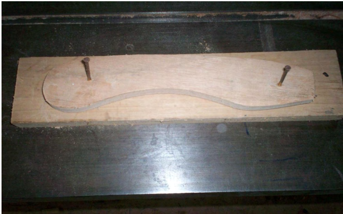
Figure 3.13 A Picture showing jig placed on a shaping sample.
