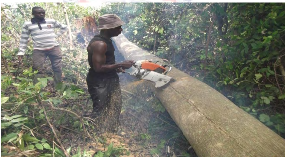
Figure 3.2 Picture of Chainsaw operator crosscutting a tree into three logs each of length 2.5m.
