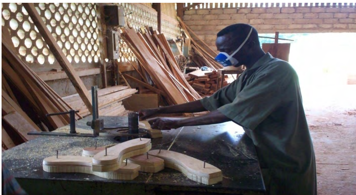
Figure 3.15 A picture showing technician performing actual shaping operation using a Spindle moulder.
