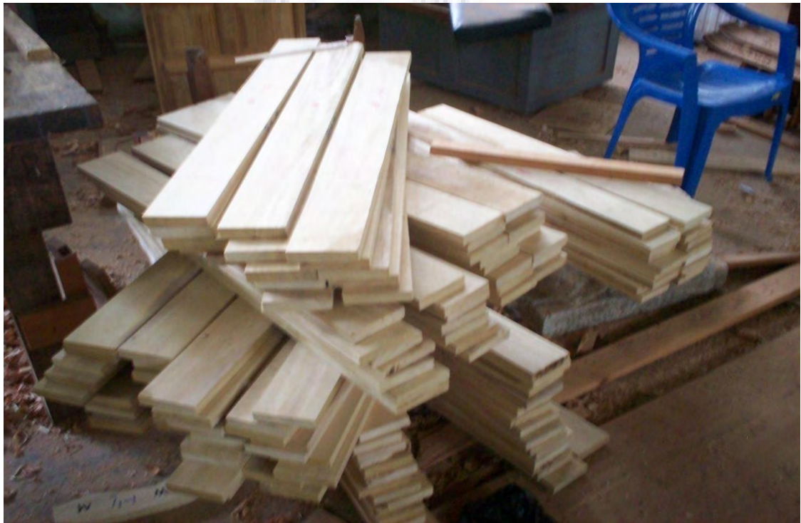
Figure 3.17 Picture showing planed specimens to be used for sanding test.
