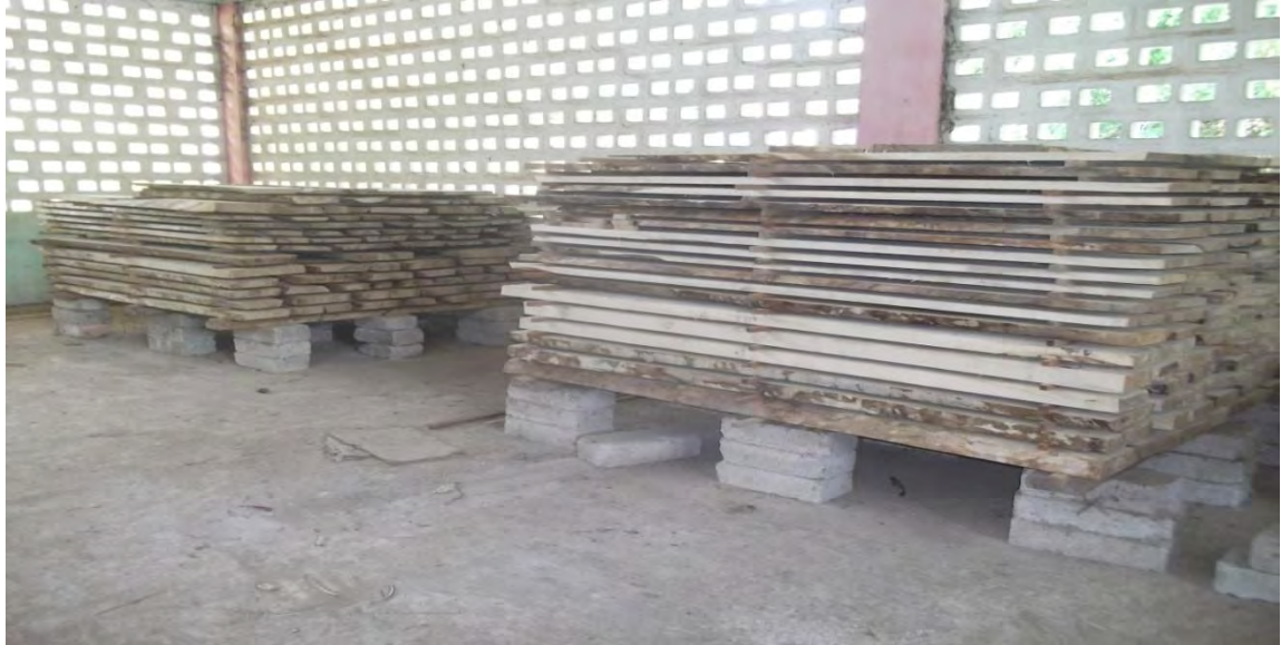
Figure 3.5 Picture of stacked boards from Daboase and Abofour under a shed to be air dried.
