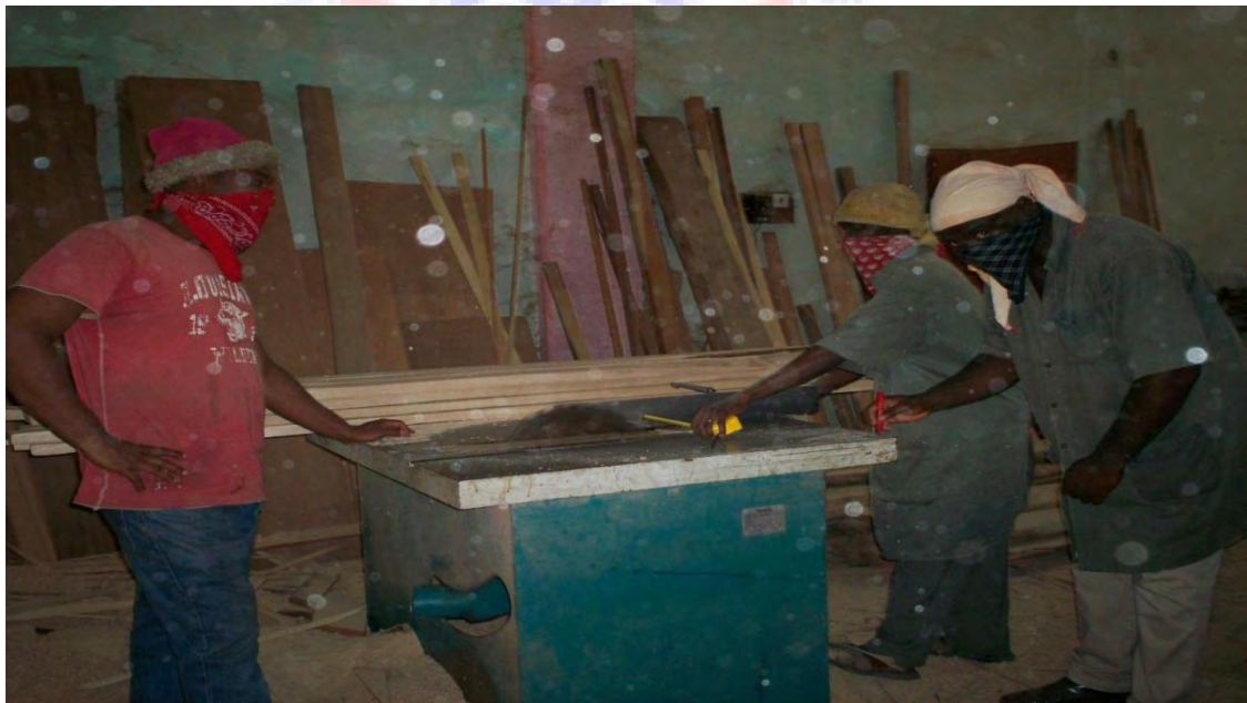
Fig.3.6 A Picture of wood workers sawing boards into required sample sizes using the cross cut machine
