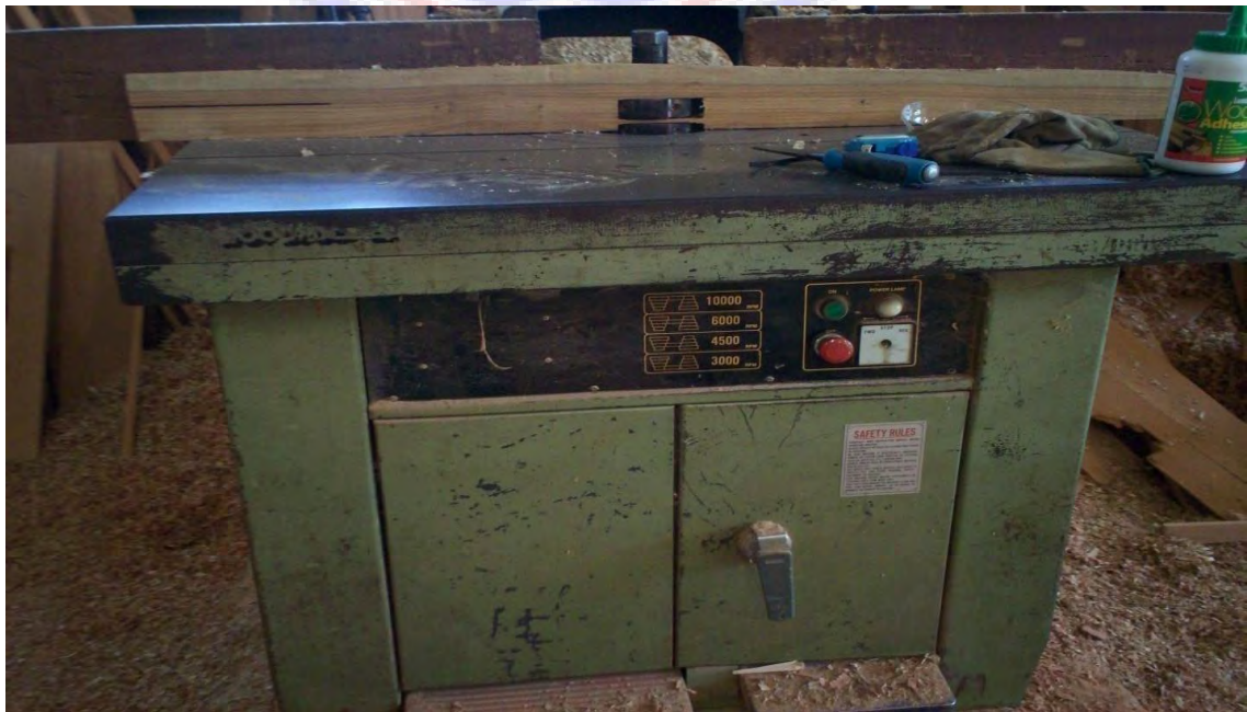
Figure 3.14 A Picture showing Spindle moulder used for the shaping test.
