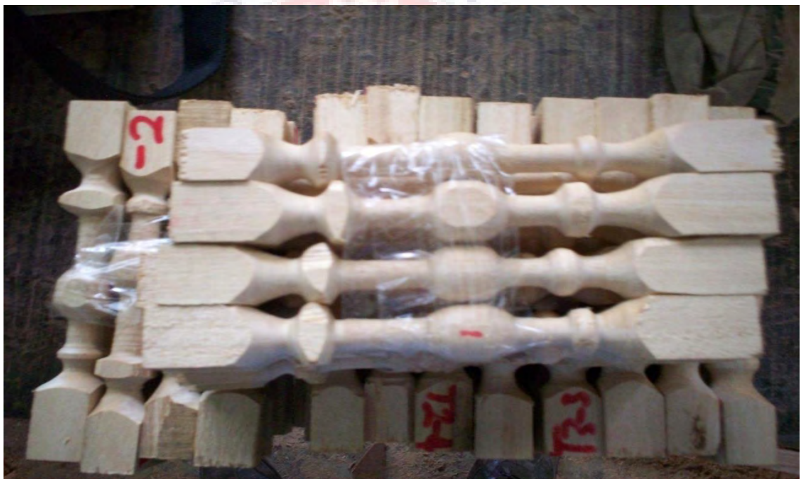
Figure 3.11 A Picture of turned specimens.
