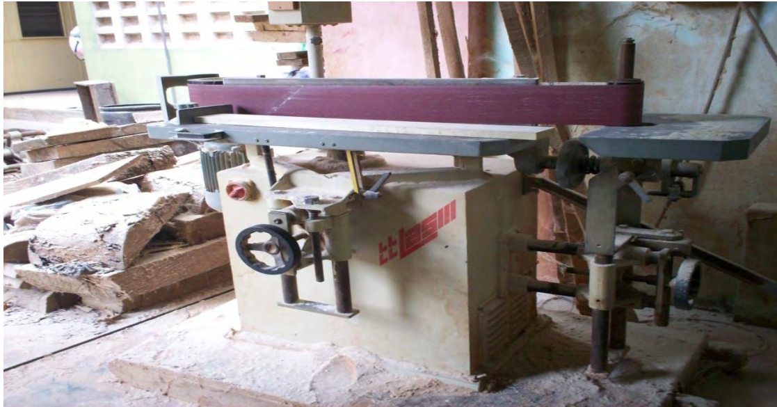
Figure 3.18 A Picture showing ttLasIII belt sander used for the sanding test.
