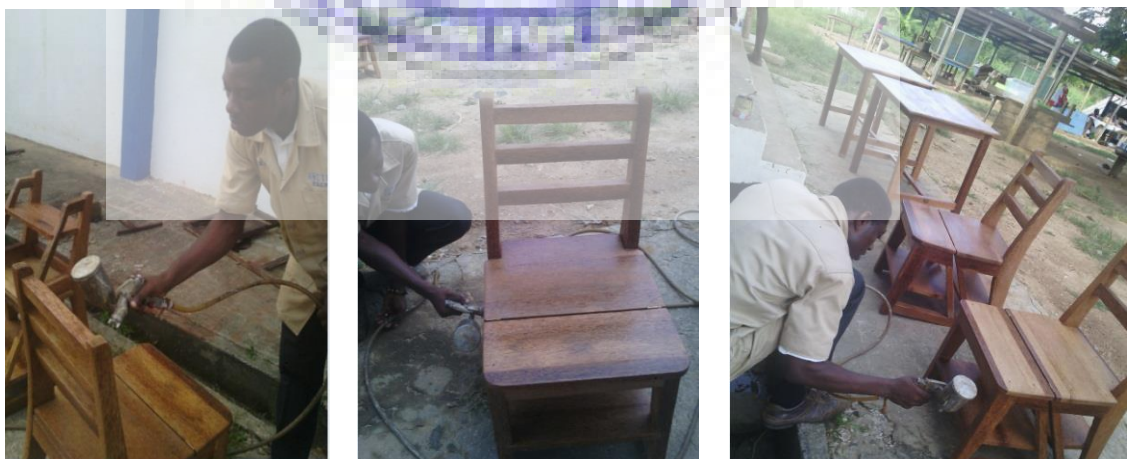
Figure 20: Application of final coating material. Source of photo: Researcher
