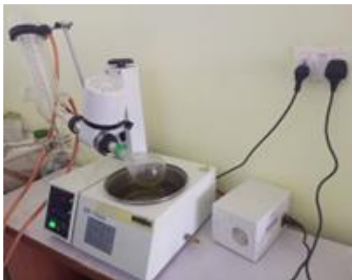
Fig.3.3. Rotary evaporator used to concentrate the ethyl acetate extract.
